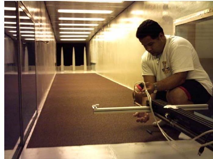
Test section: 17 m x 1.7 m x 1.7 m
