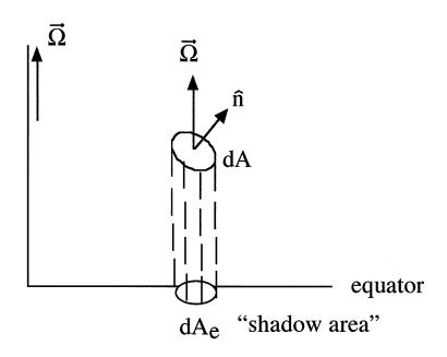
$$dA_e \equiv \frac{\vec{\Omega}}{\Omega} \cdot \hat{\mathbf{n}} dA \quad [\frac{\vec{\Omega}}{\Omega} \text{ and } \hat{\mathbf{n}} \text{ are unit vectors}]$$
