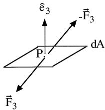
$\vec{F}_3$  is force exerted across dA <u>by fluid pierced by</u>  $\hat{e}_3$  <u>on fluid on other side</u>.  $-\vec{F}_3$  is force exerted across dA by fluid pierced by  $-\hat{e}_3$  on fluid on other side.
