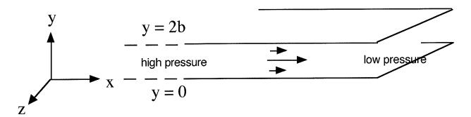
Need to impose <u>impermeability cond</u><sup>n</sup> <u>at plates</u>: no flow <u>normal</u> to plates. Automatically satisfied in this case:
