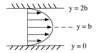
Verify that u is max at centerline. Define  $y_{\text{max}}$  by:  $\frac{du}{dy}\Big|_{y_{\text{max}}} = 0$ .
