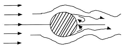
Friction important in a thin boundary layer (b.l.) adjacent to solid boundary. Can get boundary layer separation downstream (in the lee) of solid object: slow flow near bdry erupts into main flow and leads to a wake of eddies (vortices) and turbulence in the lee. Friction is important in b.l. (next to object) and in wake. But outside of b.l./wake region, friction is not important.
