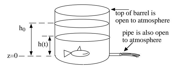
Initial height of free surface (air/water interface) is  $h_0$ . Height of free sfc at time t is h(t). Cross-sectional area of barrel is A Cross-sectional area of pipe is a (a << A)
