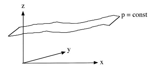
As long as we're on an isobaric sfc,  $\delta p = 0$ . Can move arbitrary increments  $\delta x$ ,  $\delta y$  in x, y directions but then we must also move a definite amount  $\delta z$  in z direction to stay on sfc.
