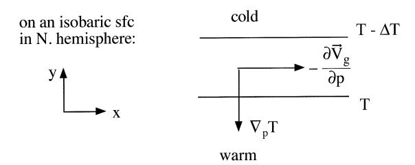
So in this case if geostrophic wind vector is westerly at surface, it intensifies with <u>height</u>. If geostrophic wind vector is easterly at the surface, it weakens with height, then reverses (i.e., becomes westerly), then intensifies with height.
