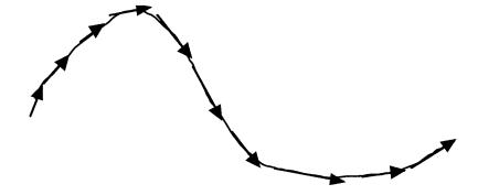
A streamline is constructed at a fixed time (snapshot). In general, it does not give history of parcel motion but <u>streamlines and trajectories do coincide if flow is in a steady state.</u>
