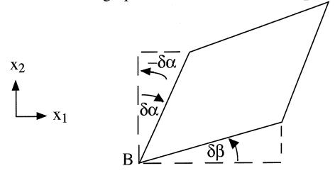
"Average" or "local" angular velocity about x<sub>3</sub> axis through B is:
