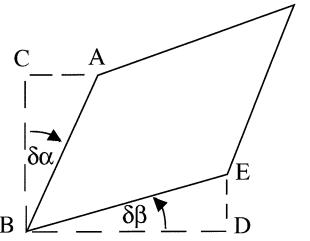
So rate of shear strain is:  $\lim_{\delta t \to 0} \frac{\delta \alpha + \delta \beta}{\delta t}$
