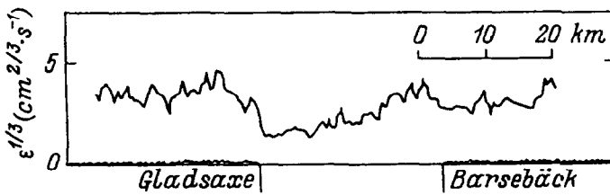
Fig. 3. Dissipation rate of turbulent energy \epsilon over Øresund and surroundings at 270-m height of 5 June 1984 (from Gryning, 1985).
