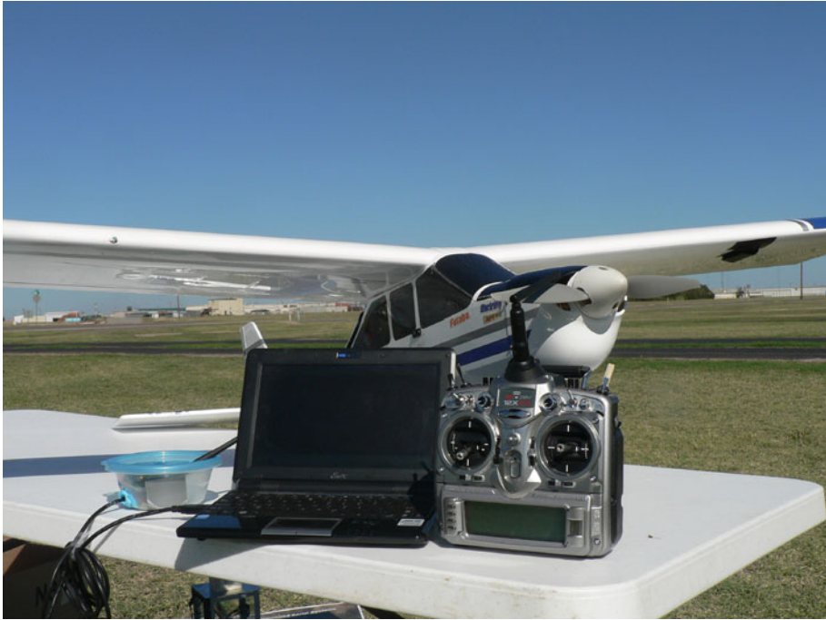
Fig. 1 Photograph of the SMARTSonde, the radio controller, and the ground control station (GCS)
