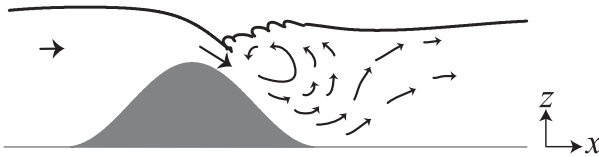
FIG. 1. Schematic diagram of the flow in a “reverse roller.”
