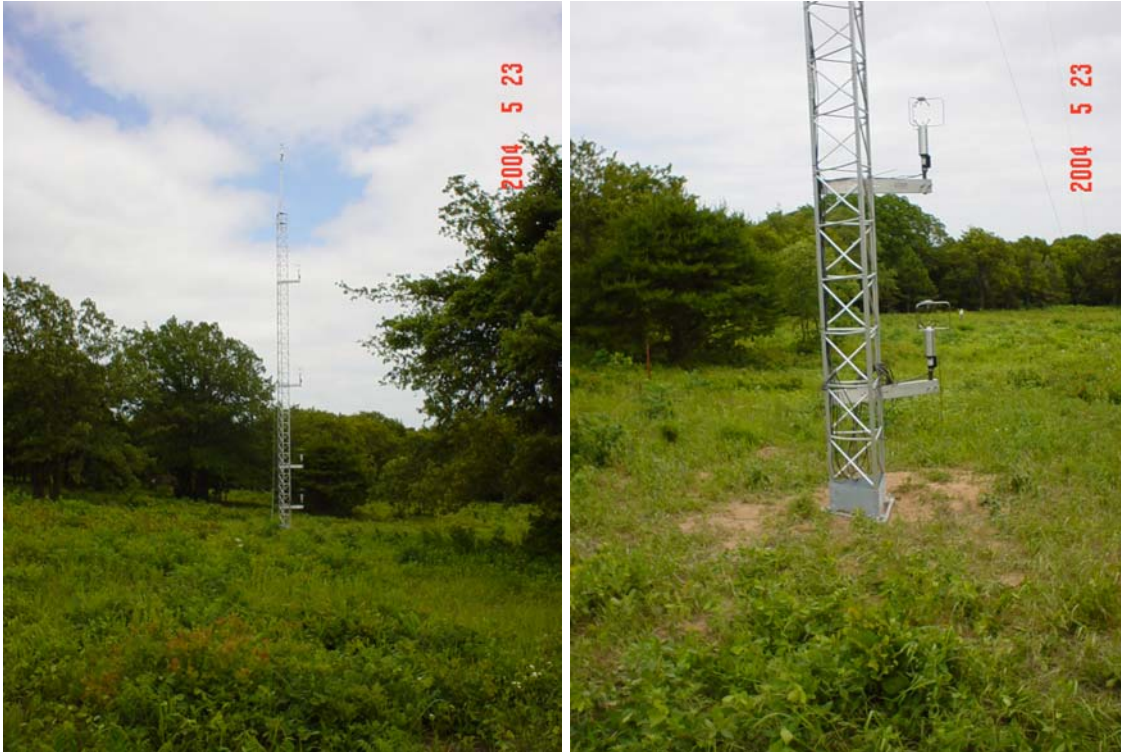
Fig. 7: Photos of the Micronet tower with 5 levels of sonic anemometer measurements.
