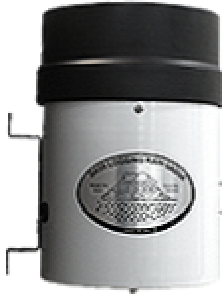
Fig. 6: Photo of the Onset's Data Logging Rain Gauge
