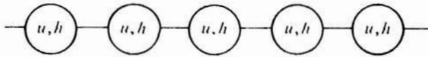
Figure 1.1 A grid with two dependent variables that are both carried at every grid point.
