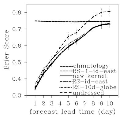
Figure 5. Brier scores (BS) for the undressed, new kernel dressed, RS-10d-globe dressed, RS-1-id-east dressed and RS-id-east dressed CCM3 ETKF 500 hPa zonal wind ensembles from 1- to 10-day lead times. The BS from the sample climatology is also shown. The vertical solid and dashed lines are the standard errors of BS calculations with given samples for the new kernel dressed and undressed ensembles, respectively. See text for further details.
